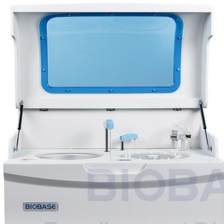
Reaction Tray 37±0.2°C, real-time monitor.
