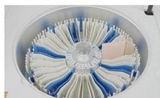
Reagent Tray 2~8°C cooling for 24 hours.
